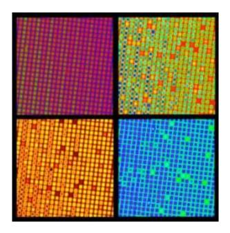
False-color images of the "fingerprints" of molecular iodine, each taken under different experimental conditions using a NIST frequency brush created with an ultrafast visible laser. The squares within each frame reveal the frequency and intensity of light from individual "bristles" of the brush. The variation in the colors reveal where the iodine absorbs specific optical frequencies. Credit: S. Diddams/NIST
