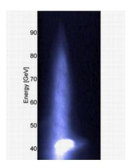
The blue streak in this photograph shows the dramatic gain in energy made by some of the electrons in a bunch after passing through plasma (ionized gas). The white spot shows the electrons in the bunch that generated the plasma to propel the other electrons to double their energy, to 85 billion electron volts (GeV). The electrons can be photographed because they emit blue light as they pass through air. Credit: SLAC
