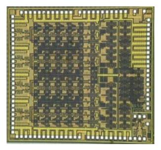
This radar chip, operating in the Ultrawideband range and made from pure CMOS, may help rescuers find lving victims trapped in rubble by detecting heartbeat and respiration. Credit: USC Viterbi School of Engineering
