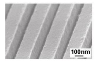
Shown is a scanning electron micrograph of the grooves in the high-indexcontrast sub-wavelength grating developed by UC Berkeley researchers. Credit: Image by Michael Huang, UC Berkeley
