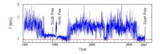
Variations of the coronal temperature measured with the SWICS instrument on board ESA-NASA's Ulysses from December 1990 to January 2007. Solar wind flow from coronal holes is characterized by high solar wind speed (700-800 kilometres per second) and low coronal temperature (1 - 1.3 million Kelvin). Credits: R. von Steiger and G. Gloeckler
