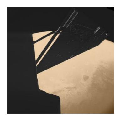
Stunning image taken by the CIVA imaging instrument on Rosetta's Philae lander just 4 minutes before closest approach at a distance of some 1000 km from Mars. A portion of the spacecraft and one of its solar arrays are visible in nice detail. Beneath, an area close to the Syrtis region is visible on the planet's disk. Credits: CIVA / Philae / ESA Rosetta
