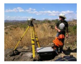
Graduate student Richard Styron makes a final visual check of a GPS antenna setup over a newly installed geodetic benchmark near Laurel Galan, Nicaragua. This is one of several new sites installed near the boundary of the Nicaraguan Depression to investigate the transition from the seismically active forearc sliver to the stable Caribbean plate. Photo by Henry Turner.
