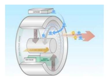
Georgia Tech's new engine uses a novel electric and magnetic field design that helps better control the exhaust particles. Ground control units can then exercise this control remotely to conserve fuel. Credit: Georgia Tech
