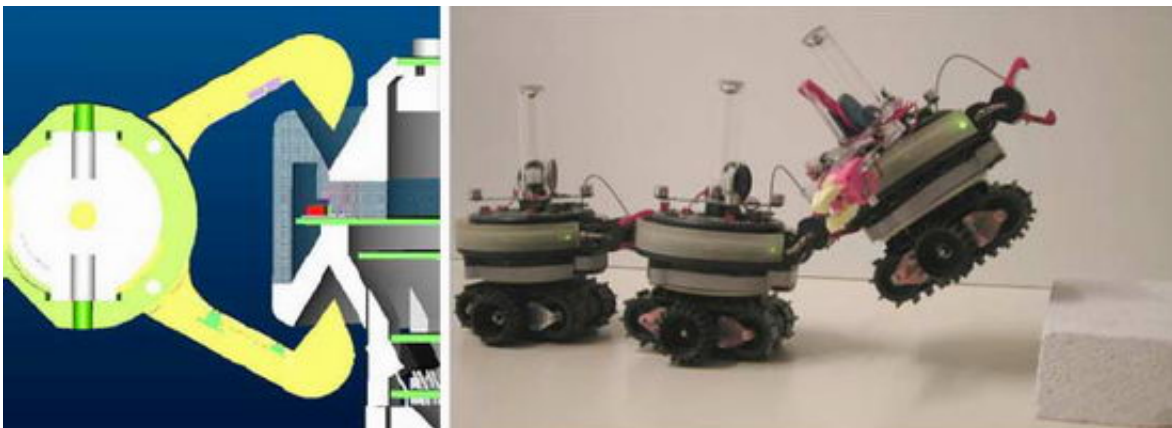
(Left) The rigid gripper used to connect s-bots. (Right) Three s-bots form a swarm-bot that can climb a step. Credit: Groß et al. ©IEEE 2006.
