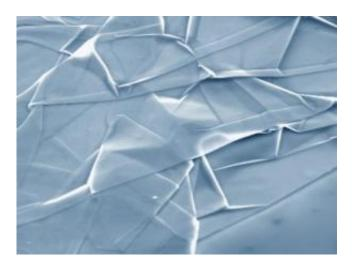
This image is a scanning electron microscope micrograph of a strongly crumpled graphene sheet on a silicon wafer. The lateral size of the image is 20 microns. The Si wafter is at the bottom right corner of the image. Credit: Courtesy of the Foundation of Fundamental Research on Matter, the Netherlands
