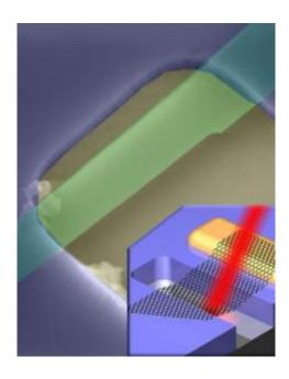
Colorized SEM image of a suspended graphene resonator. (inset) Schematic of the resonator. The graphene is in contact with a gold electrode that can be used to electrostatically actuate the resonator. A red laser is used to detect the motion of the resonator by laser interferometry. Credit: Arend van der Zande and Scott Bunch
