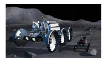
In this artist's concept, a pair of lunar astronauts embarks on an extra-vehicular science mission onboard an unpressurized rover. Aided by their robotic work assistant traveling at their side, the astronauts will be able to achieve scientific and exploratory objectives never before possible. All equipment will be carried on the two vehicles, thus streamlining mission complexity and allowing the two crewmembers to concentrate all their efforts on the mission at hand. Image Credit: NASA
