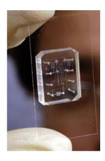
Johns Hopkins researchers helped invent this microfluidic chip, which features tiny channels and chambers in which they can conduct experiments on small clusters of cells. Credit: Will Kirk/JHU
