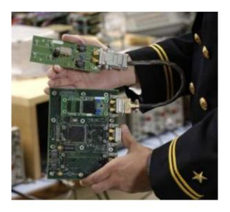
The microdosimeter instrument consists of small sensors connected to an electronics board, shown here without the casing. Spacesuits integrated with this technology can warn astronauts at the onset of an elevated exposure event, assess risk, and help crews determine safe locations during these periods. Source: National Space Biomedical Research Institute
