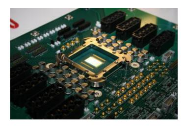
This board houses Intel's 80-Core Teraflops Research Chip. The board contains working silicon and it is the world's first programmable chip to achieve teraflops performance while consuming very little power. Credit: Intel
