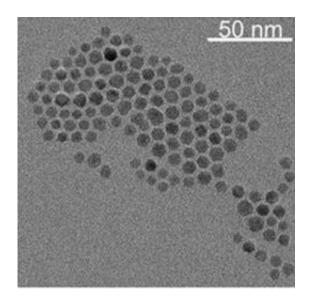
Electron microscopy of the magnetic nanoparticles. Credit: IMEC
