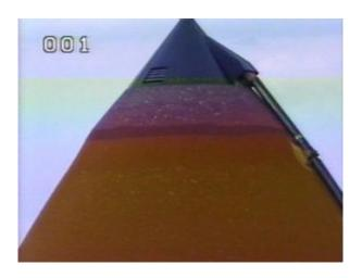
A strong thunderstorm with hail damages Atlantis space shuttle&acutes external fuel tank. A remote camera view of the external tank with hail marks. Credit: NASA/KSC
