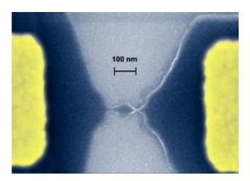
Single-electron transistors carved entirely in a graphene sheet. The central elements are so-called quantum dots allowing electrons to flow one by one. The dots are connected to wider regions (contact pads by nm-wide constrictions) that work as tunnel barriers. Credit: University of Manchester
