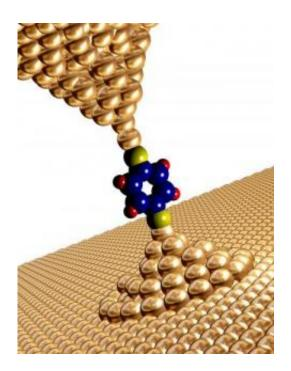
Graphic of an organic molecule trapped between two gold surfaces. When one side is heated, a current is created. Credit: Ben Utley image
