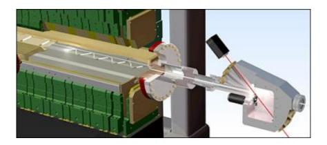
To time-stamp the arrival of each x-ray pulse, researchers use an electro-optic crystal (green) placed next to the electron beam (white) in the linear accelerator just before the beam produces x-rays. A laser (red) probes changes in the crystal to measure the exact time the beam passed by. This image was created by Jean Charles Castagna, SLAC.
