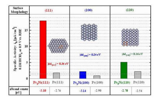
Diagrams show the influence of the surface morphology on the kinetics of a cathodic fuel cell reaction. Credit: Argonne National Laboratory
