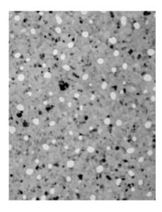
Electron microscope image: pores in the membrane are white. Credit: University of Rochester
