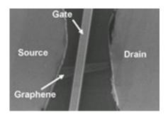
In the scope of his innovative project ALEGRA the AMO nanoelectronics group of Dr. Max Lemme was able to manufacture top-gated transistor-like field-effect devices from monolayer graphene.
