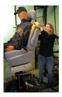
Purdue mechanical engineering doctoral student Janette Jaques attaches a sensor to a car seat headrest mounted to a hydraulic shaker. As the seat is shaken, sensors record vibration data used to validate results from a computational model that simulates the vibration. The goal is to silence rattling and squeaking noises in a car's headrest and other components, a major source of consumer dissatisfaction that automakers would like to eliminate. Credit: Purdue News Service photo/David Umberger
