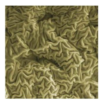
Wrinkled hard skin on polymer surface induced by focused ion beam. The wrinkles are hierarchical with the primary wavelength of 465 nm. Photo courtesy / Moon et al.
