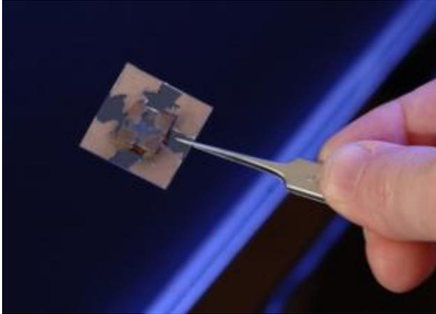
Since the late 1990s, Lauterbach and Snively have been developing a method to make extremely thin polymer layers on surfaces. The film covering the surface of these metal samples is at least 1,000 times thinner than a human hair. Photo by Kathy F. Atkinson
