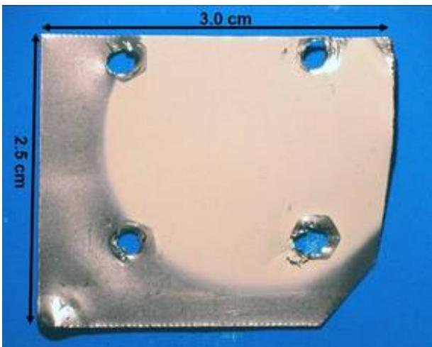
This photo shows an ultra-thin polymer film of fumaronitrile, which formerly was believed to be 'unpolymerizable,' on a tantalum foil. The film is circular due to the shape of the window where ultraviolet light is emitted into the vacuum chamber during the film deposition process. Photo courtesy of Lauterbach Laboratory, University of Delaware
