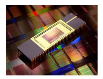
Samsung Electronics announced that it is now sampling its 16-gigabit (Gb) NAND flash memory with customers – the first NAND flash using 50 nanometer process technology.
