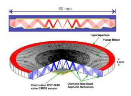
Above: cross section of an eightfold imager. Below: cut-out view of the same imager. The blue lines illlustrate the path the light follows as it moves from aperture to light sensor. Credit: UC San Diego
