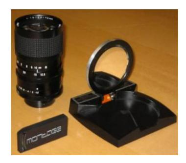
Top left: conventional 35mm camera lens Right: Montage Phase-1 folded imager (descibed in the Feb 2007 Applied Optics paper) Bottom left: Montage Phase-2 folded imager (only mentioned in the current paper. Will be descibed in future publications). Credit: UC San Diego
