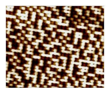
False-color image of 50-nanometer cobalt-palladium nanodots made with a magnetic force microscope provides both topographic and magnetic profiles. The darker dots are magnetized in the up direction (representing 1 in binary code) and the lighter dots are pointing down (representing 0). Credit: NIST
