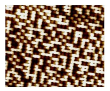
False-color image of 50-nanometer cobalt-palladium nanodots made with a magnetic force microscope provides both topographic and magnetic profiles. The darker dots are magnetized in the up direction (representing 1 in binary code) and the lighter dots are pointing down (representing 0). Credit: NIST
