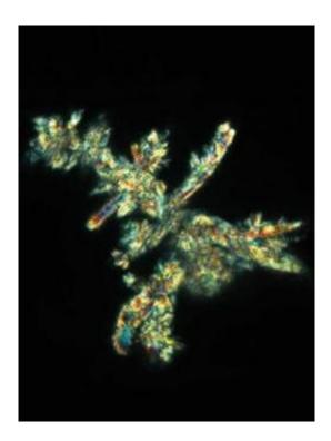
A zoomed view of a bright, ordered domain in the nanocomposite. Upon heating to temperatures above 120 degrees Celsius, the bright domains disappear. But upon annealing the material at 60 degrees C for 68 hours, the bright domains reappear. Image width=0.18 mm. Image courtesy / Gareth McKinley Lab
