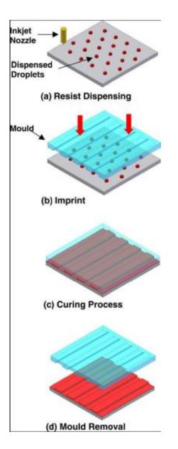
In dispensing nanoimprint lithography, liquid droplets on the surface of a silicon wafer are pressed into a pattern, which quickly hardens to form the desired circuitry. Credit: Stephen Chou/Princeton University
