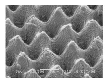
The double structure (pillars with ripples on them) is clearly visible in this polymer surface. Credit: University of Twente
