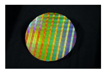
Intel 300mm 45nm wafers similar to the SRAM test wafer shown here will be used to make the company&acutes next generation, 45nm Intel Core 2 Duo, Core 2 Quad and Xeon families of processors – codenamed Penryn. Credit: Intel
