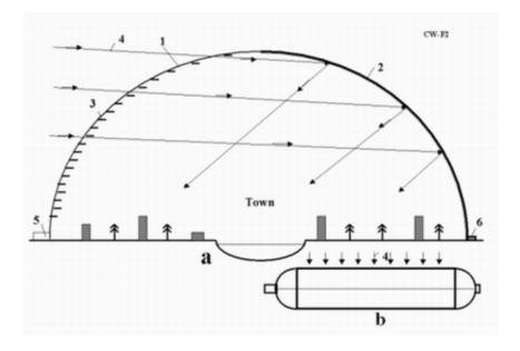
Inflatable dome for cold, high-latitude regions on Earth. The main figure (a) shows a cross-section of the suggested biosphere, and the small figure (b) shows a top-down view. The important components are labeled: a thin, transparent double film on the sunlit side (1), a reflective cover on the shaded side (2), control louvers (3), the entrance (5), and an air pump/ventilator (6). The direction of the Sun is indicated by beams of light (4).
