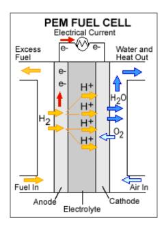
PEM fuel cells consist of electrodes containing a platinum catalyst and a solid polymer electrolyte. By splitting hydrogen molecules at the anode, and oxygen molecules at the cathode, PEM fuel cells generate an electrical current with only heat and water as a by-product. Credit: Berkeley Lab
