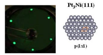
The green dots in this Low Energy Electron Diffraction pattern for a single crystal of Pt3Ni(111) reveal a tightly packed arrangement of surface atoms that wards off platinum-grabbing hydroxide ions and boosts catalytic performance. Credit: Berkeley Lab
