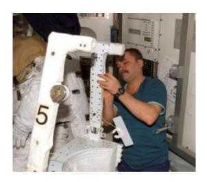
Expedition 14 Flight Engineer Mikhail Tyurin works with an Extravehicular Mobility Unit spacesuit in the Quest Airlock of the International Space Station. Image credit: NASA
