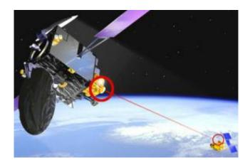
Carrying three payloads plus a number of experiments, Artemis (Advanced Relay and Technology Mission Satellite) has been designed to test and operate new telecommunications techniques. The L-band mobile payload allows two-way voice and data communications, via satellite, between fixed Earth stations and land mobiles - trucks, trains or cars - anywhere in Europe and North Africa. Credits: ESA-J.Huart
