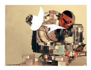
LOLA telescope assembly, as fitted to aircraft used in the Artemis laser link trials. Credits: Astrium
