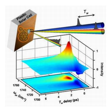
A plot of the wavelength of emitted infrared light vs. the time delay of the light emission provides information about the path of an electron within a plastic solar cell. This information about how the cell makes an electric current from light will lead to improvements in the efficiency and usable lifetime of solar cells. Credit: Penn State
