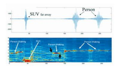
This graphic illustrates data analysis from a Sandia in-house customized sensor, showing advanced pattern recognition identifying an SUV compared to a person. The large sophisticated sensor — complete with onboard GPS, compass, local and long-haul radios, ditigal signal processor, and video capabilities — is supplemented by small, low-cost, low-power, commercially available sensors. Credit: Sandia National Laboratories
