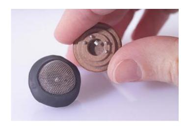
This improved hydrogen gas sensor was developed by a Russian organization with PNNL technology assistance. It was licensed to Apollo Sensor Technology in 2006. The sensor could be used in a variety of environments where hydrogen gas is present, to detect leaks. Credit: PNNL
