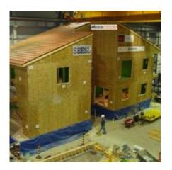
A two-story, 1,800 square-foot, fully furnished townhouse was built and placed inside the lab on two moveable, piston-powered shake tables, among the largest of their kind in the United States. Engineers and researchers jolted, shook and rattled the house in a series of five mock earthquakes that grew in size and magnitude. Credit: Texas A&M University
