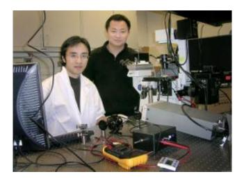
Chang Lu, at right, a professor of agricultural and biological engineering, and graduate student Jun Wang run a test on their microfluidic chip that fuses cells. A growing research technology, cell fusing is vital in studying stem cells, creating clones and finding disease antibodies. Credit: Purdue Agricultural Communication photo/Tom Campbell
