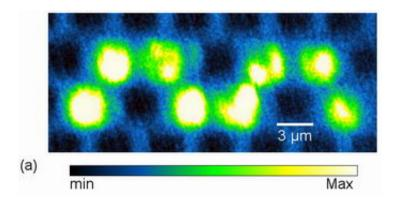
Francesca Intonti and her colleagues created this curved waveguide by filling the pores in photonic crystals with a water solution, which provides a "leak" in the band gap and permits the flow of light. Credit: Intonti et al.
