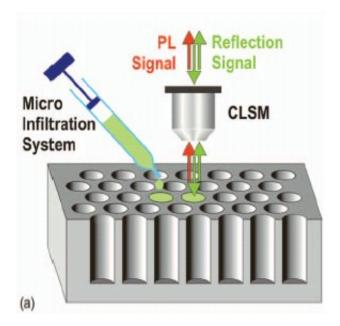
The microinfiltration system enables liquid to enter pores in the photonic crystals in drops of less than 1 femtoliter, or a million billionth of a liter. Infiltration is monitored by a confocal laser scanning microscope (CLSM) mounted on top of a standard microscope. Credit: Intonti, et al.
