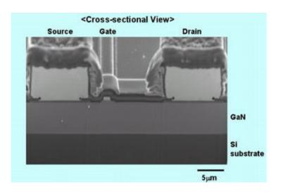
Normally-Off GaN Power Transistor With Low On-State Resistance. Credit: Panasonic
