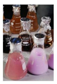
These beakers contain various samples of carbon nanotubes or the nanomaterial  $C_{60}$ , also known as 'buckyballs,' mixed in water stabilized either by surfactants or natural organic matter. Credit: Photo by Gary Meek
