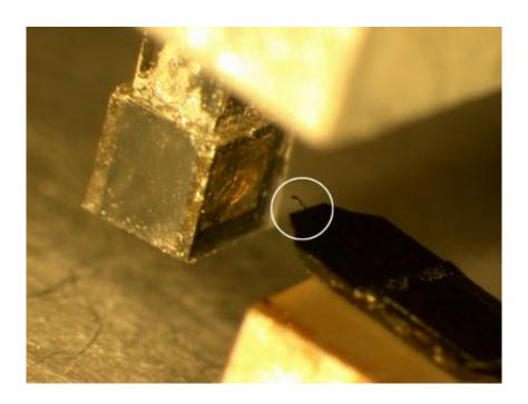
Micro-cantilever experiment demonstrating magnetic coupling of mechanical motion to atomic spin. The approximately 200-micrometer cantilever (circled) has a tiny magnetic particle on the free end. Rubidium atoms are confined in the cubic vapor cell to the left. Credit: Ying-Ju Wang, NIST
