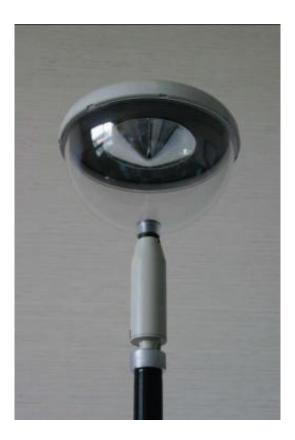
Photograph of a wide-angle "catadioptric" lens with a lipstick-shaped bullet camera on a pole. Credit: Gyeong-il Kweon, Honam University, South Korea, and colleagues
