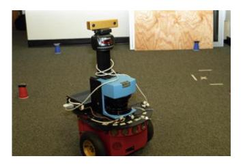
Aristo, the Washington University robot, uses sensor networks to avoid simulated "fire" - red cups - while navigating near "safe" areas, which are blue cups. Credit: WUSTL
