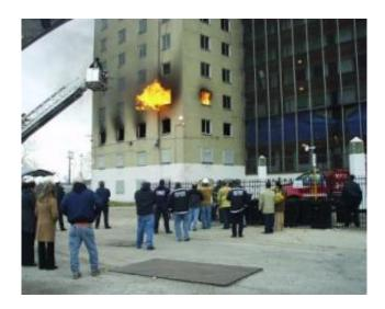
Members of a research team watch flames erupt from an abandoned Chicago apartment building during a Nov. 10 test of positive pressure ventilation in high-rise fires. Red truck (lower right corner) is a mobile ventilation system blowing air through the front door of the test building to keep the corridors and stairwells passable, while forcing the fire outside. Credit: NIST
