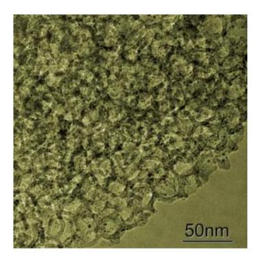
An electron microscopic image shows gold nanoparticles staining enzymes (tiny dark spots) trapped inside functionalized mesoporous silica chambers (larger blobs). (Color added.) Credit: Pacific Northwest National Laboratory
